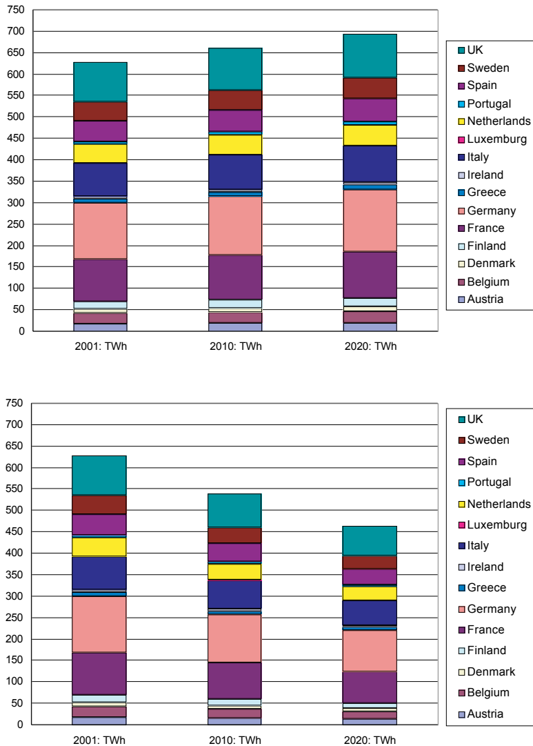
Figure 12.3: The energy use of the public sector by Member State of the EU. Above is the baseline scenario (a) and below is the strong energy efficiency scenario (c). Summarizing the outcomes of the scenarios, the energy use of the public sector in 2020 shows a +10%...-20% change compared to 2001 (excl. the worst case scenario). Related to the total national heat and electricity uses in the Member States, this means in practice a +1.5... -2% change from the reference level 2001.
